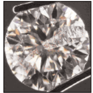
There is an obvious contrast of this uneven fracture on this diamond traveling all the way through its culet.
